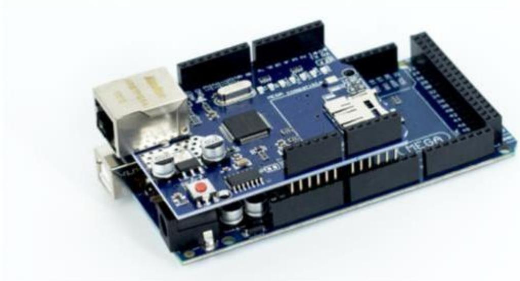
Figura 9 – Shields Ethernet
